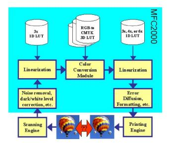
Figure 1. Simplified flowchart of the color copy operation in ViewAhead's MFC2000 MFP controller chip. The color LUTs are optimized to achieve the best color image quality in the copied image.
