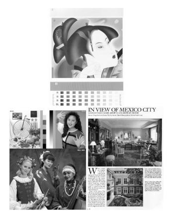
Figure 4. The three images used in the experiment. Top: 11, a test target provided by an MFP manufacturer. Left: 12, a composite image created using SCID24 images, printed on a continuous-tone Fujix Pictography printer. Right: 13, a mixed-content page taken from a magazine.
