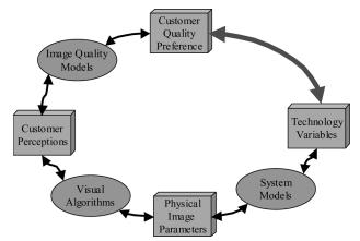
Figure 3. The Image Quality Circle. The desired mapping between the technology variables and the customer's perception of quality is sought to be found through a three-level approach — system models, visual algorithms, and image quality models. Adapted from Engeldrum.<sup>23</sup>
